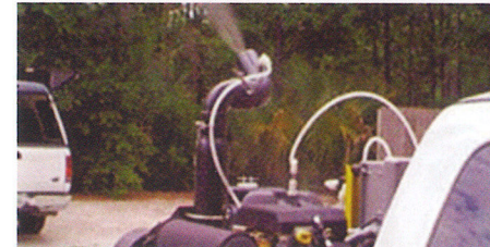
Outdoor ULV with truck mounted ULV machine.
